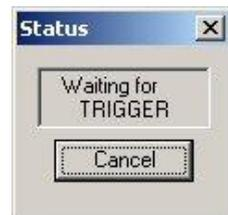
As soon as the second trigger is seen, the Waiting for Trigger message will change to Reading Data and the trace will start to appear on the screen. Immediately after the trace is completed, the whole screen will be redrawn with the trace shown centrally on the chart according to the reference standard that has been selected – unless the View option Raw Data has been selected (see next section).
