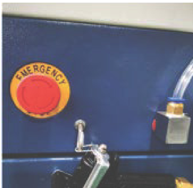
Emergency Stop Button
