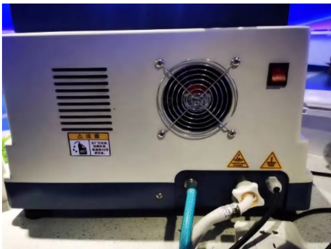
Electrical & Water Cooling System
