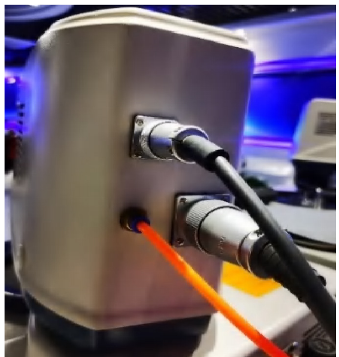
Grinding Head with Electricity & Air Pressure
