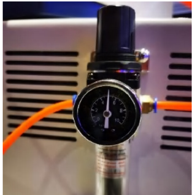
Air pressure Meter
