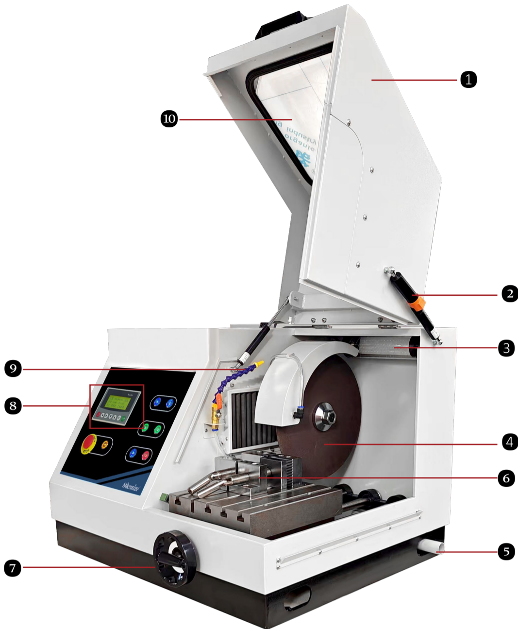
2. Protective lighting lamp 4. Cut-off wheel 5. Outlet pipe port 6. Clamp 7. Handwheel 8. Screen and buttons 9. Coolant nozzle 10. Transparent observation window
