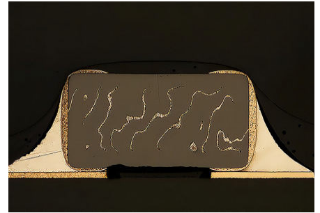
Capacitor tin plating height detection
