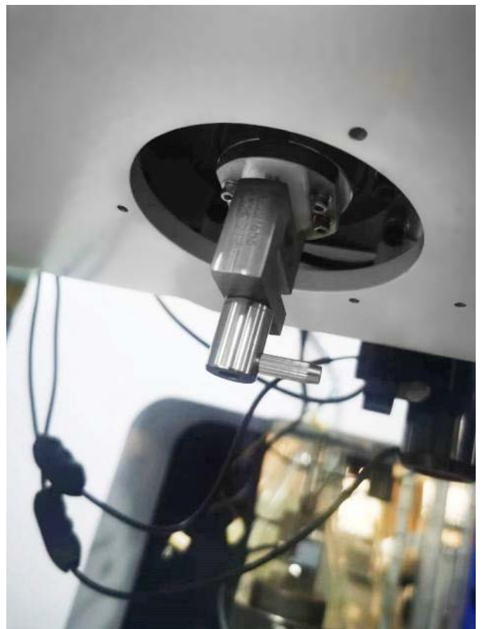
Load Cell above Indenter
