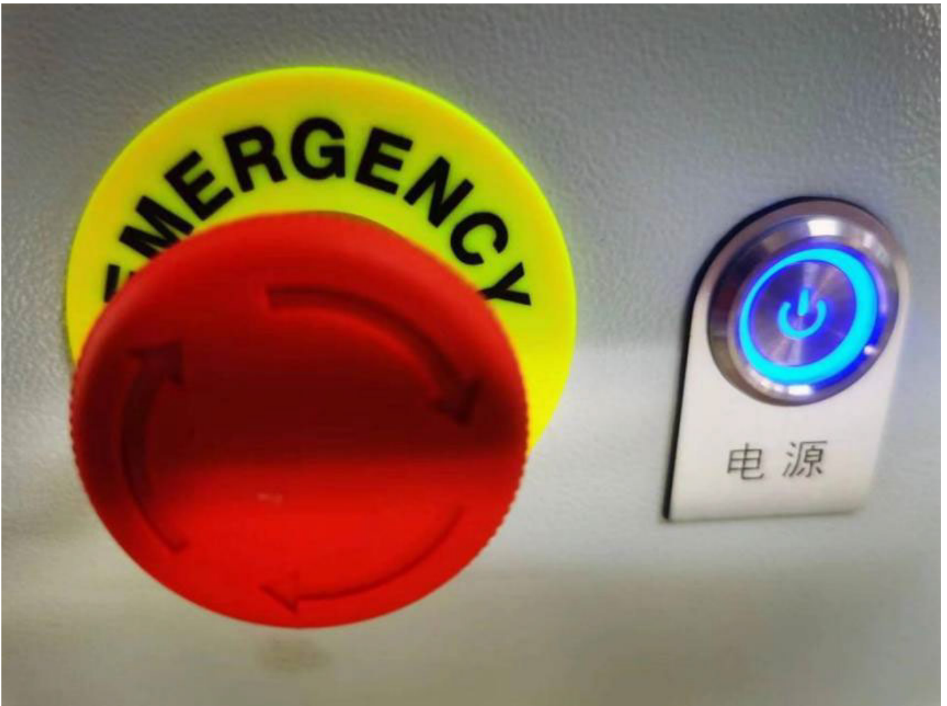
Power on/off and Emergency Stop Button
