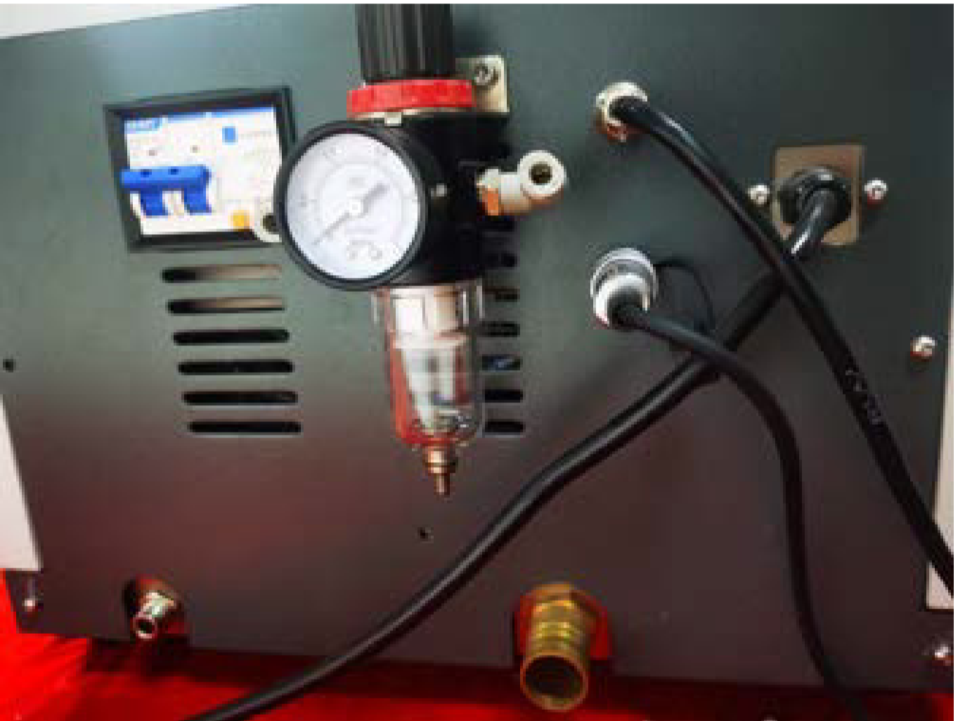
Water Cooling/ Electric / Air Pressure System
